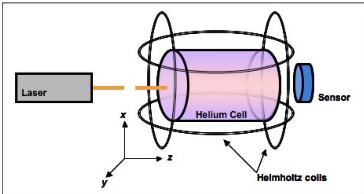
*Figure 1: Partial diagram of Vector Helium Magnetometer. Pictured is the 1083nm laser traveling along the optical axis of the cell, two of the three pairs of Helmholtz coils, the glass cell of metastable Helium, and the magnetic field sensor. Not pictured is the computer control system and the RF supply that ignites the cell.*
