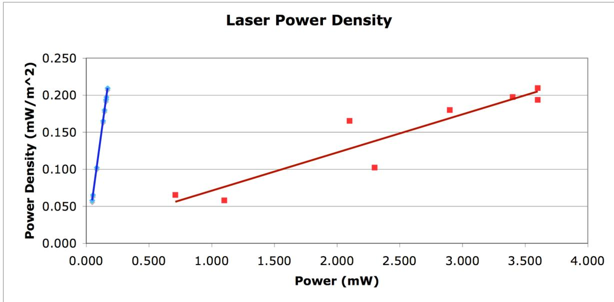
*Figure 2:* Graph of Power Density vs. Laser Power of the laser beam entering the helium cell. The line on the right side of the graph represents the correlation between beam power and power density of the expanded beam when measured without the lens cap aperture. The line of the left side of the graph represents the correlation between beam power and power density of the expanded beam when measured through a lens cap with a 1mm aperture.
