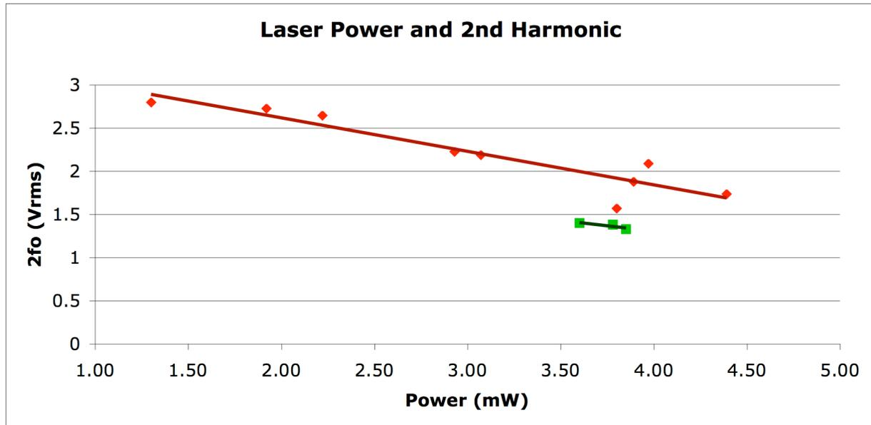
Figure 3: Graph of Magnitude of 2nd Harmonic vs. Laser Power. The upper line represents the power and 2nd harmonic magnitude relationship for the expanded beam, the lower line represents the same relationship for the unexpanded beam.
