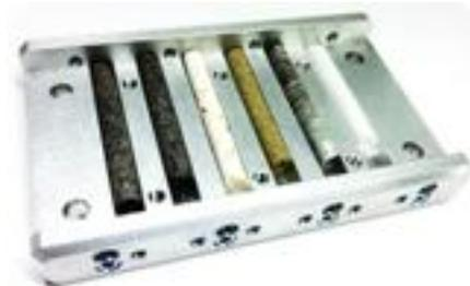
Figure 4. A clamshell holding the bare rock cores.
