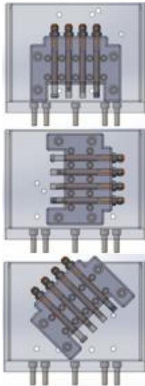
Figure 7. The rock cores mounted onto the vibe mount in vertical, horizontal, and diagonal orientations. The tests are conducted in one orientation at a time.
