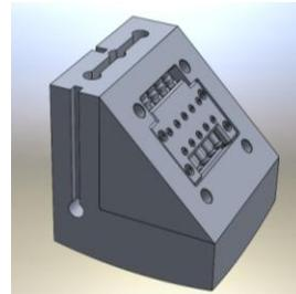
Figure 3. The CAD model of the shock block showing the third set of rock cores set in the diagonal orientation.
