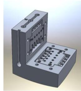
Figure 2. The inside of the shock block with the rock cores in the horizontal and vertical orientations.
