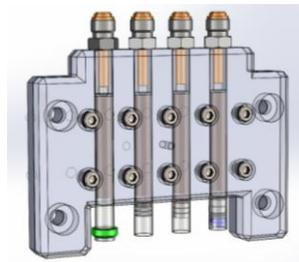
Figure 5. The top half of the clamshell and test tubes are shown transparent.
