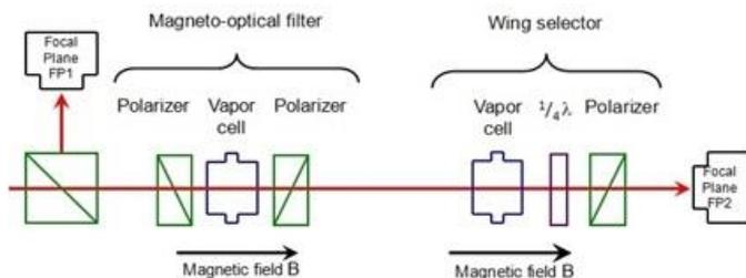
Figure 1: Previous Design Schematic
