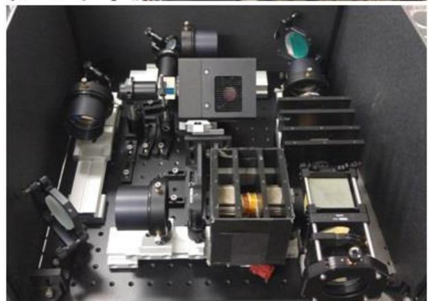
Figure 5: a) Doppler Imager without enclosure and back mount. B) Doppler Imager with enclosure.
