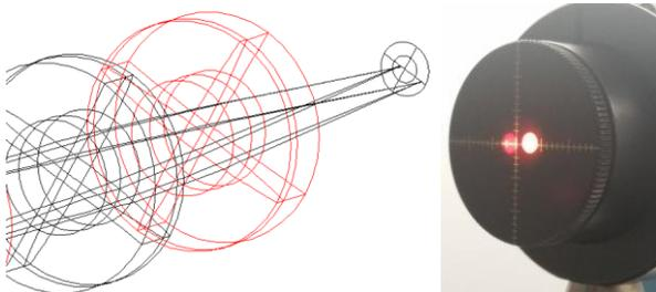
Figure 4: Image of sun modeled in Winlens 3D (left); real image (right)
