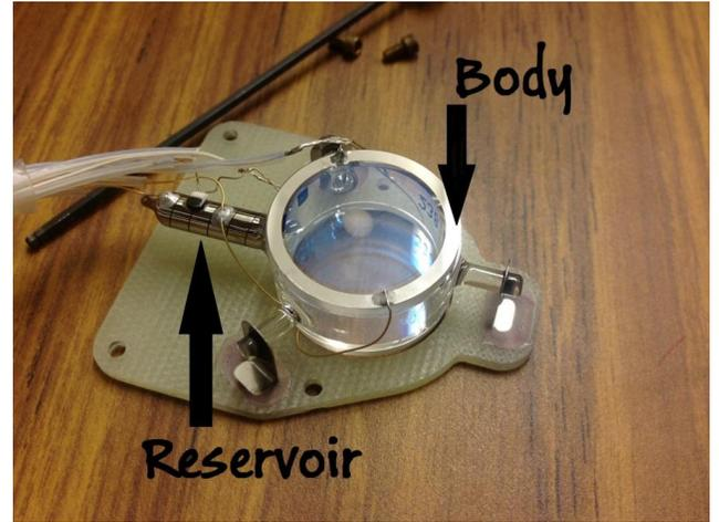
Figure 5: Magneto-optical filter with body and reservoir denoted.
