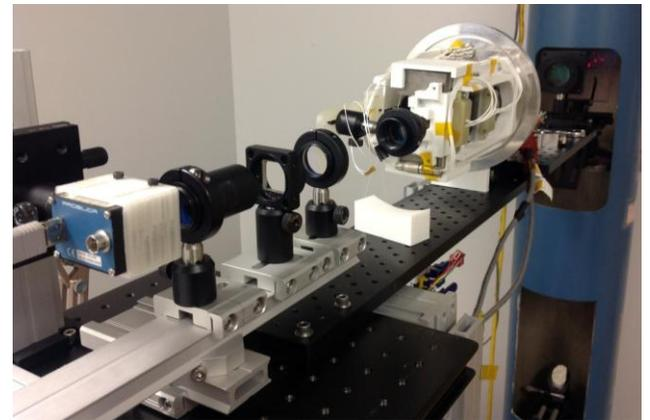
Figure 6: Full optical layout of instrument; aperture in background, CCD with 3D printed holder in foreground
