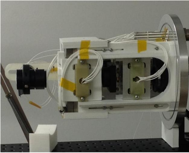
Figure 3: 3D printed MOF mount within vacuum chamber.
